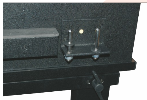
Bass side parts with different plug-in points for beams
